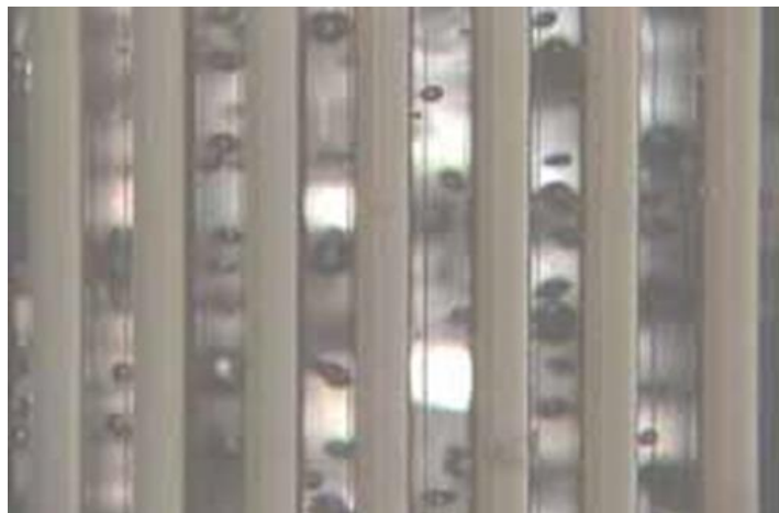
Figure 4: Fixed spacing between each membrane cartridge provides efficient air scour
